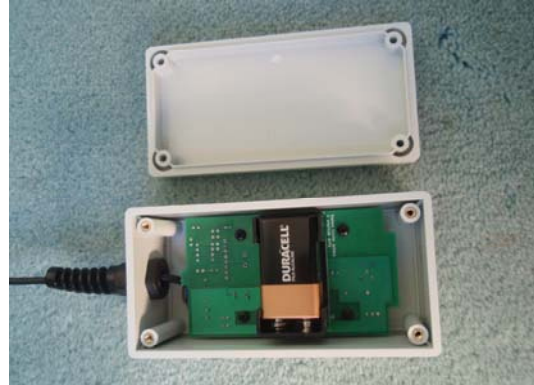
Figure 8 Back cover removed to show battery.
